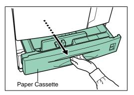
2 Remove the jammed paper while taking care not to tear it. If the paper has been torn, remove all the scraps from the inside the printer.
